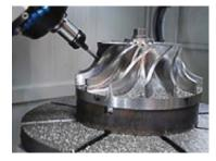
CNC machines produce precision parts by cutting, drilling, and grinding parts used in the vast majority of all manufactured products. CNC machinists make adjustments to the machine to control speed, material feed, and path of the cut, as well as make sure the machines are set up properly, working well, and producing quality product by using a wide variety of precision measuring instruments and inspection techniques.
